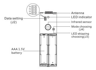
**Infrared sensor:** Used to detect infrared signal of human body radiation, please don't touch the lens with your hand and keep it clean.
